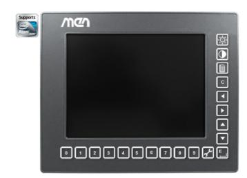
The DC13 panel PC is a rugged, fanless and maintenance-free human-machine interface (HMI) for interactive railway applications with a power consumption of less than 13 W. It is designed as a stand-alone panel and equipped with a 8.4" TFT LCD display with 20 backlit front keys with tactile feedback.
